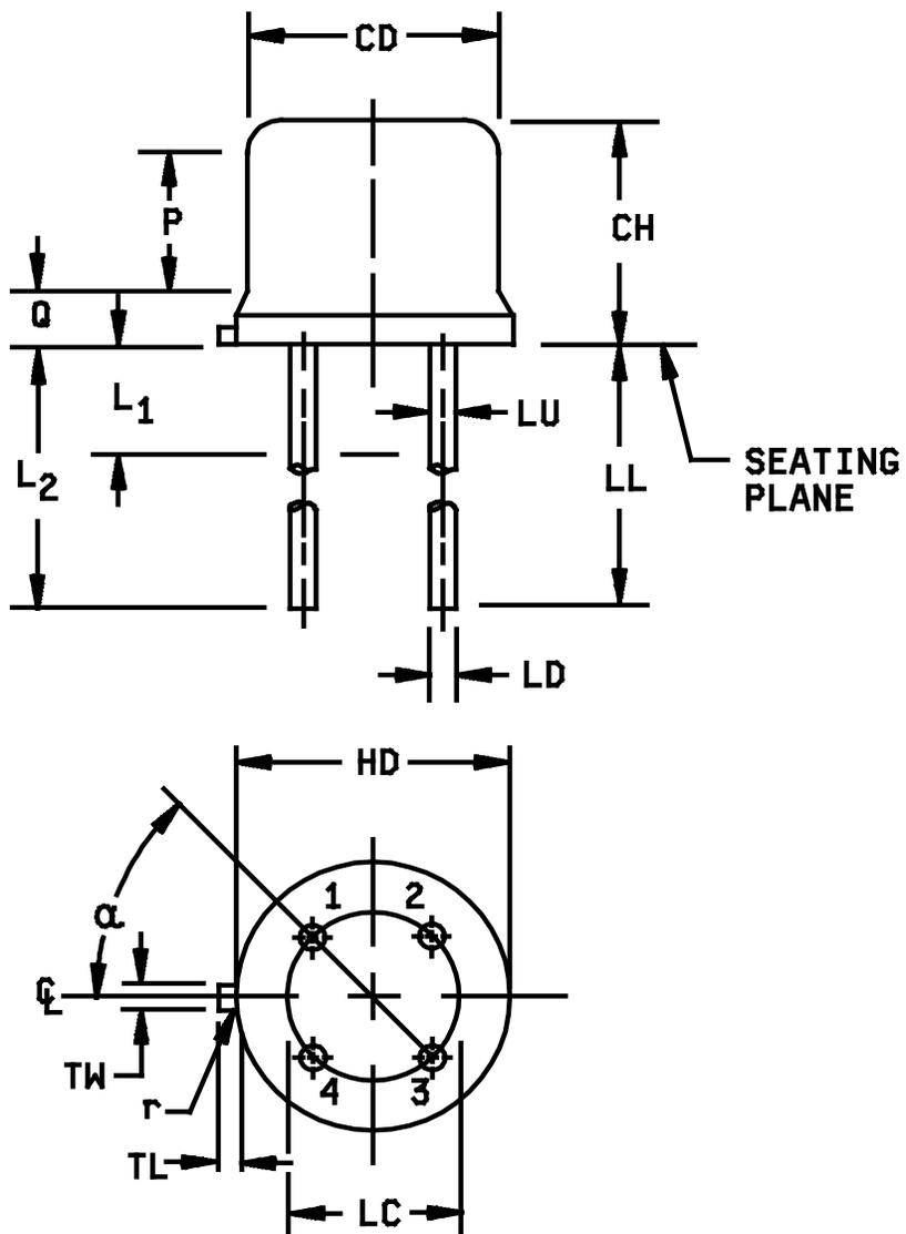
FIGURE 1. Physical dimensions of transistor type 2N4957 (TO-72).
